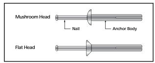
to expand. The anchor is pre-assembled with either a carbon steel or stainless steel nail. As the nail is driven into the anchor body, each half of the expansion mechanism is compressed against the walls of the drilled hole. This anchor is not recommended for applications overhead.
